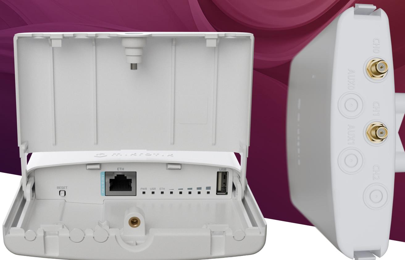
*This weatherproof board features a modern Qualcomm Maple CPU based on the ARM architecture, 256 MB of RAM, a USB port for extra storage or other needs, and a Gigabit Ethernet port with PoE-in.*
